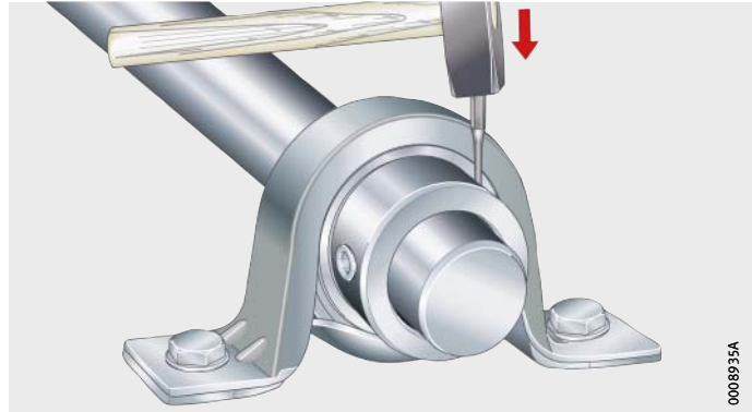
Figure 13 Tensioning the eccentric locking collar
