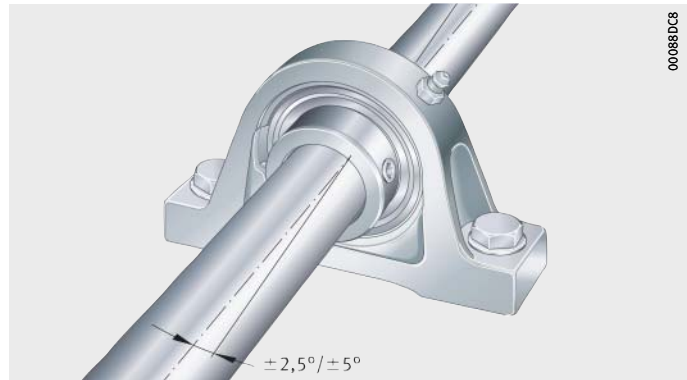
Figure 1 Compensation of static shaft misalignment
