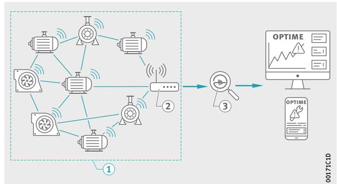
The standard version of the gateway already has an integrated SIM card for use exclusively in conjunction with the OPTIME system. If the proposed mobile phone connection is not to be used, there are other options for connecting to the Schaeffler IoT Hub, i.e. using a separate SIM card, a WiFi connection or connection via network cable.
