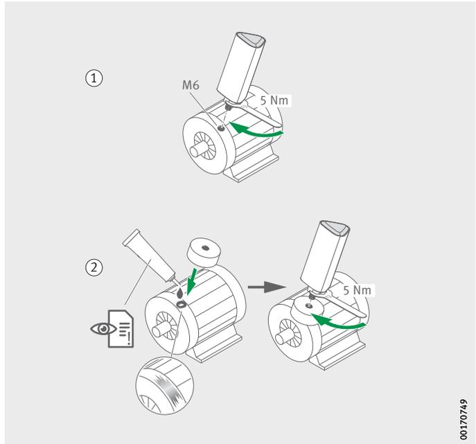
Mounting a sensor into an existing thread on the machine requires a flat surface and an M6 screw-in thread, *Figure 20*:
