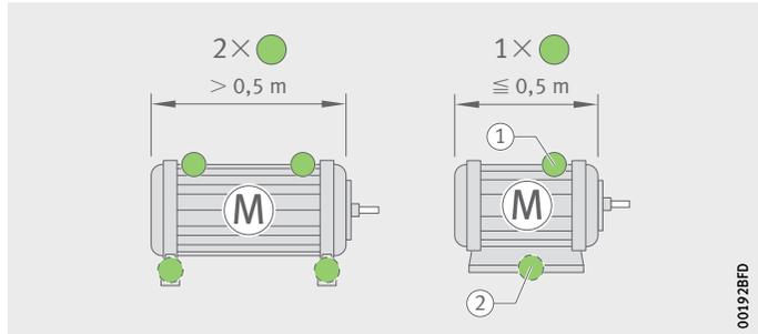
In the case of machines that are significantly larger than 0,5 m, it is recommended that at least two sensors be used so that potential damage can be readily identified. The same applies if two machine components are separated by a coupling, as in this case the vibrations cannot be transmitted adequately via the coupling.
