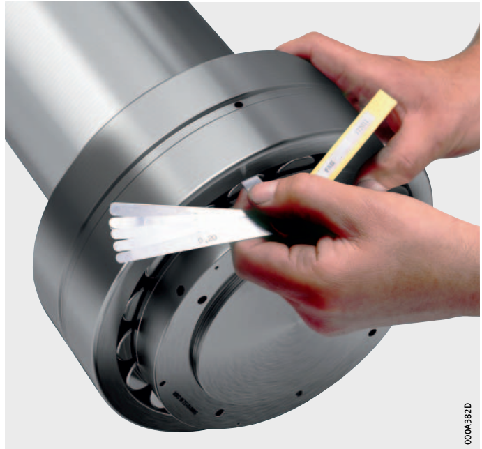
Figure 11 Measuring reduced radial internal clearance
