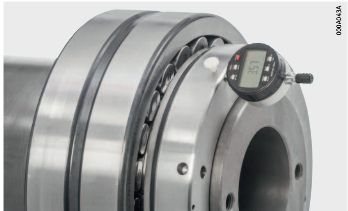
Figure 9 Measuring the axial drive-up distance
