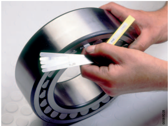
Figure 10 Measuring the radial internal clearance
